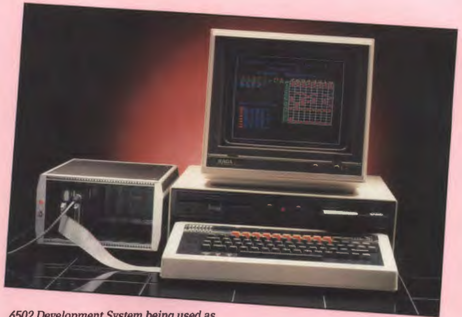
6502 Development System being used as a FILESERVER in a typical network application.
